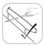
Ensure that the cutterblade is balanced. Use a screw driver with a round shaft to support the cutterblade through its centre hole. Hold the cutterblade horizontal and then release. A balanced cutterblade will remain horizontal.
